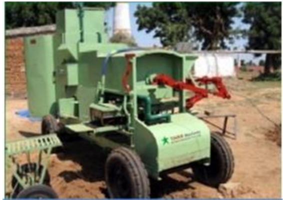
Soft mud moulding machine developed by DA Group for marble sludge and soil mixing
